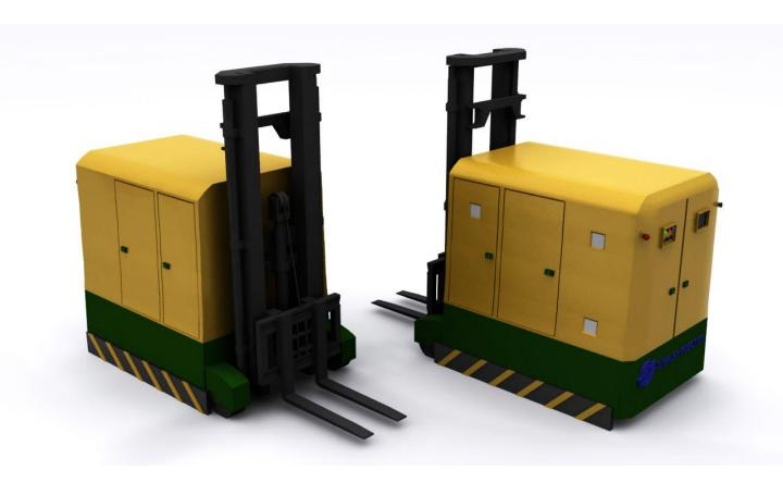
RISHABH- Fork type Automated Guided Vehicles (AGVs) are autonomous mobile robots used to transport materials from loading to unloading stations. It is a highly flexible, intelligent and versatile material handling vehicle
